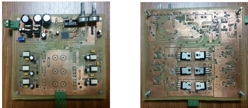
Figure 3. Designed Three-Phase Asynchronous Motor Driver Card
