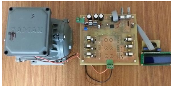
Figure 4. Three-Phase Asynchronous Motor Driver System
